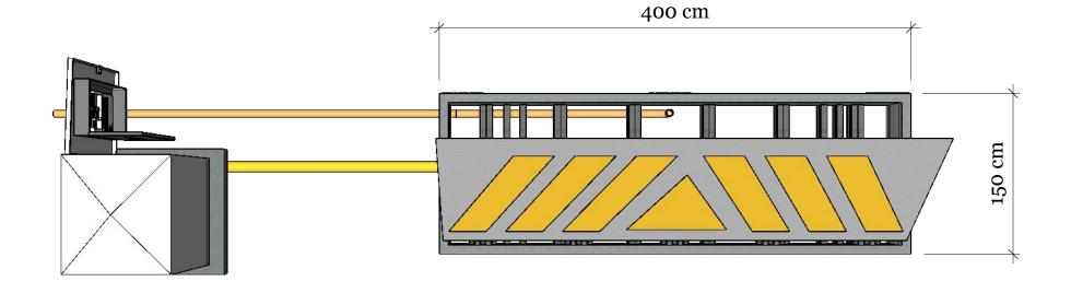
Shallow Mounted Crash Rated Wedge Road Blocker Barrier System
